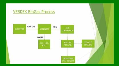
In the chart above we show our process. We take the raw gas from the digester, we remove unwanted components, such as CO2, and we compress RNG at 3,600psi. We then move the gas to a location where it can be put to use. Generally it is injected in a pipeline, used for transportation or industrial boilers.
